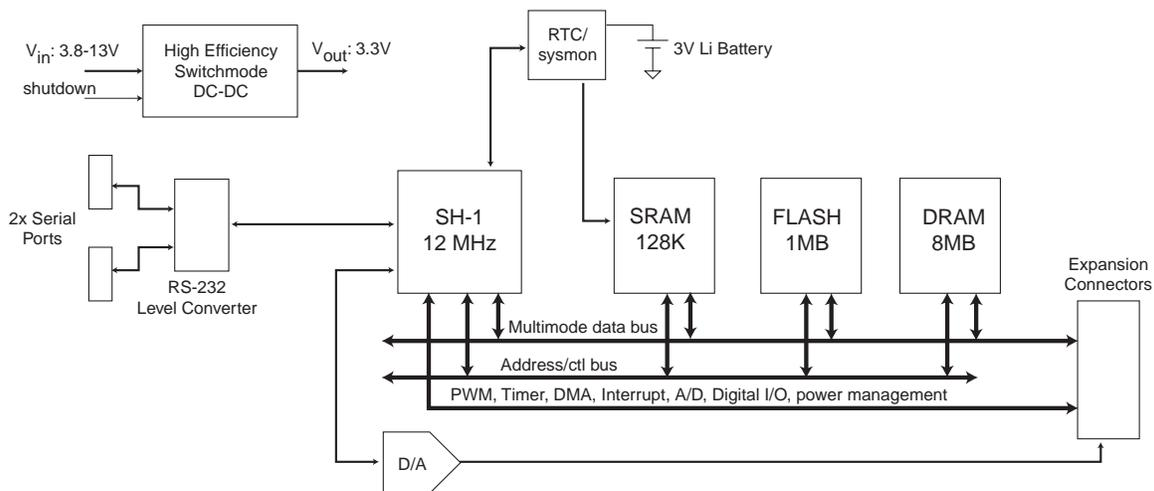
Figure 1: SH-1 Workhorse system block diagram
