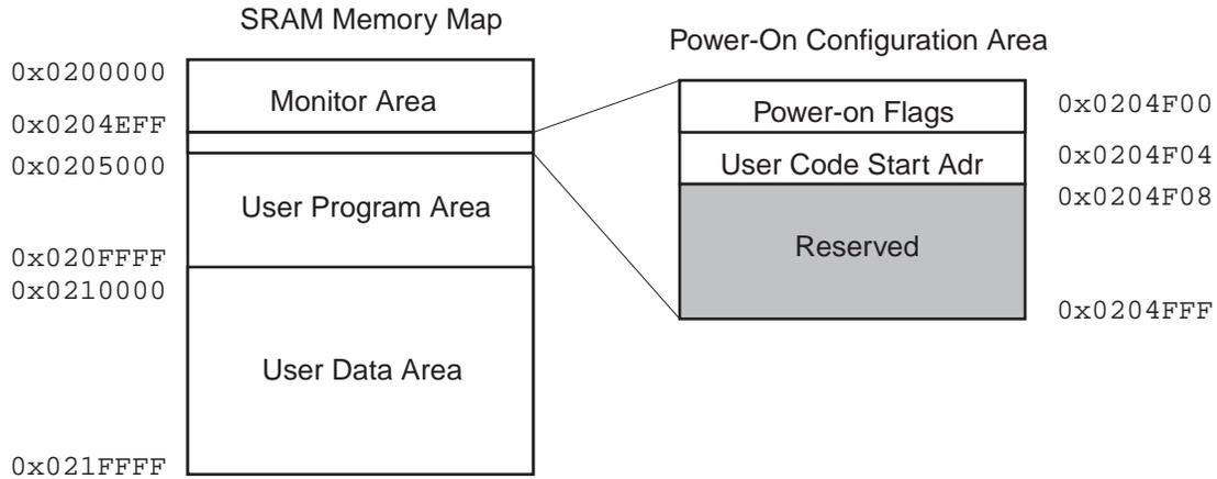
**Figure 8: Recommended SRAM footprint.**
