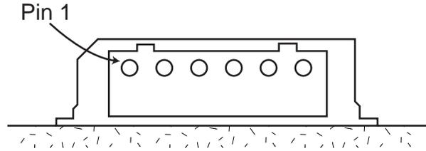
**Figure 2: Serial Connector (J1) pin 1 orientation (viewed head-on from side of board)**
