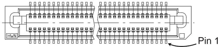
**Figure 4: J3 and J5 pin 1 location, top view of connector**
