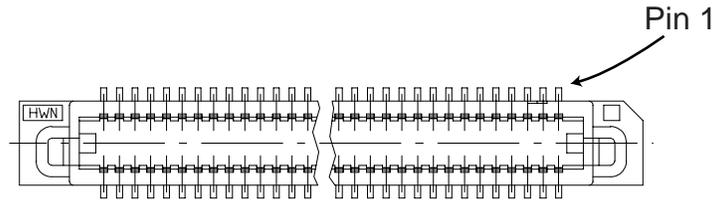
**Figure 3: J2 and J4 pin 1 location, top view of connector**
